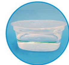
Slight deformation on flange
